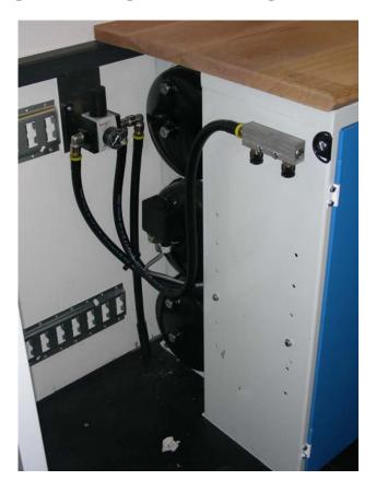
Inputs / Outputs 220 V / 430 Vac for external main power and compressed air output
