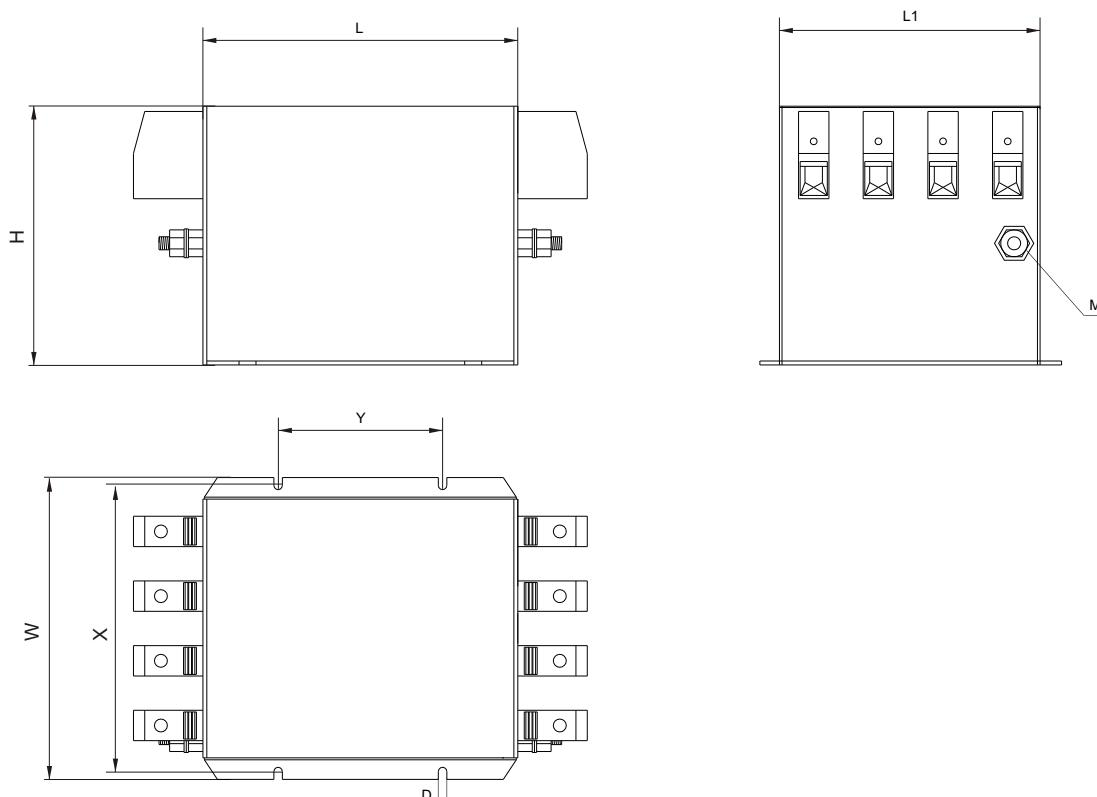
**Terminales: Faston, Bornas****Terminals: Faston, Shrouded**Dimensiones en mm.
