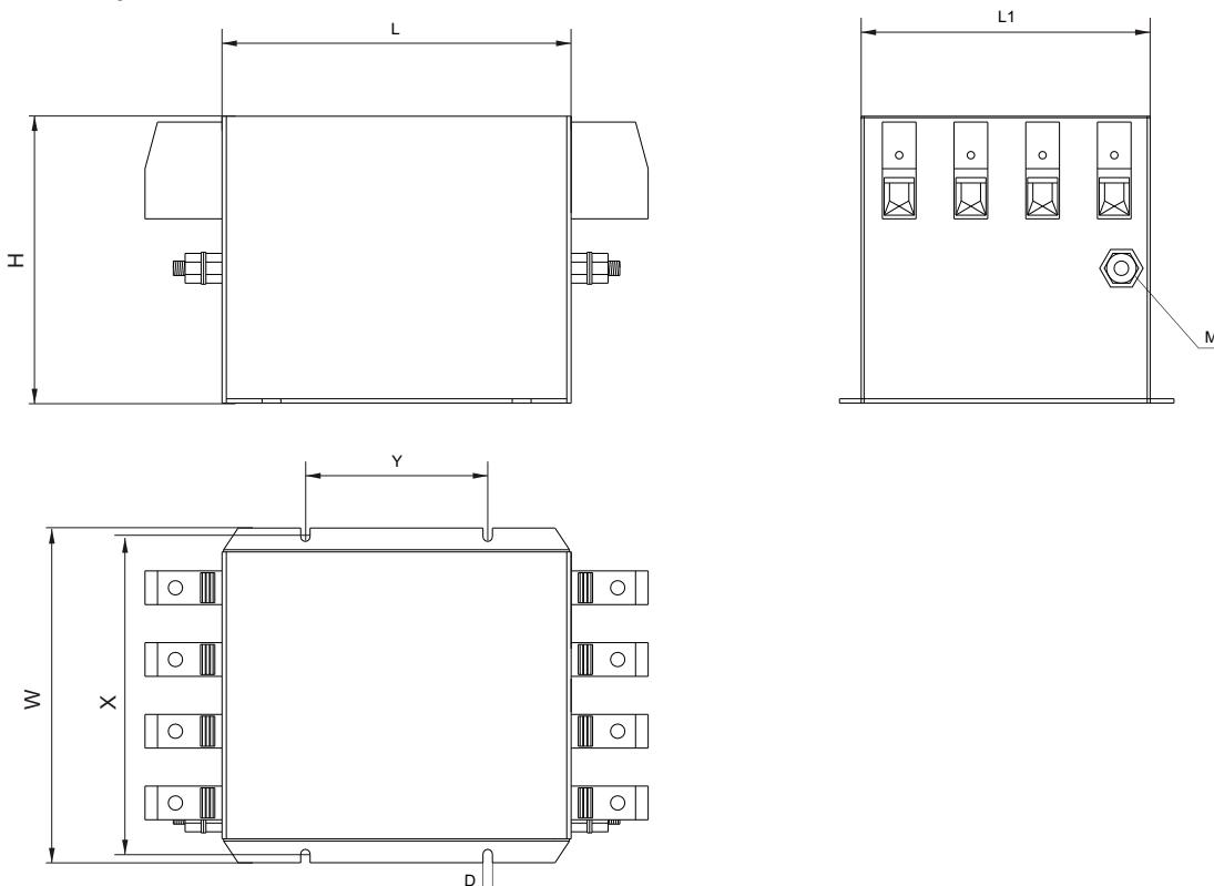
**Terminales: Faston, Bornas****Terminals: Faston, Shrouded**Dimensiones en mm.
